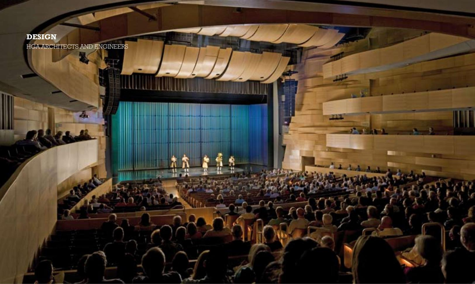
semi-trucks. The stage, 35m-wide and 15m-deep, has an adjustable proscenium frame and 60 manually controlled line sets for stage scenery, draperies and lighting. An easily accessible grid iron is 23m above the stage and the sprung wood floor has a 4 x 8m modular structurally framed trap. The 636 theatrical lighting circuits can be individually controlled by computer or remote touchscreen panels.
